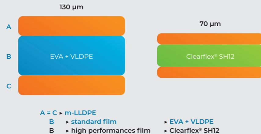
**Clearflex® SH12** is a highly innovative compound based on polyolefins having elastomeric characteristics. This compound has a perfect balance among elastic, rheological, optical and mechanical properties. Fig.1 shows (magnitude 1:15,000) the amorphous molecular structure, strongly interpenetrating between the thermoplastic and the elastomeric polymers, properly chosen and compounded.
